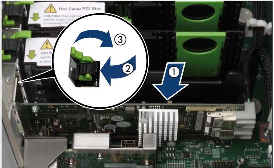
Figure 97: Inserting the Modular RAID controller
